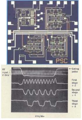
Fig. 5. Divide-by-eight gated prescaler with 2 GHz clock fabricated and tested at HP Labs in 1976.
