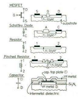
Fig. 7. The 1981 *RFIC Process* offered designers a complete set of components: MESFETs, Schottky Diodes, resistors and thin-film capacitors.
