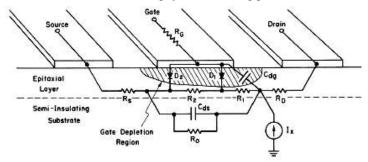
Fig. 4. The 1974 non-linear MESFET device model was based on a 2-lump approximation of the FET channel. Pinchoff was proportional to square root of gate voltage, but velocity saturation - approximated by the hyperbolic tangent function – mimicked the short-channel properties of the MESFET. This model became a key tool for subsequent IC design [21].
