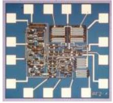
Fig. 6. The RF Signal Generation chip of 1978/79. The local oscillator tuned 2.1-2.5 GHz using on-chip tuning diodes and an off-chip inductor. The downconverted I.F. was dc - 1.4 GHz.
