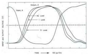
Fig. 3. The NAND/NOR logic gate showed 60ps delay with one output load, 75ps with two loads, 105ps with three loads.
